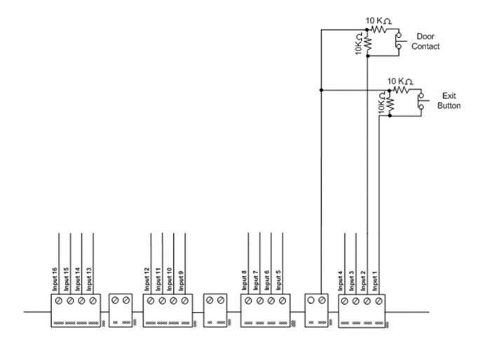
Note: Setting of this switch applies to all analog 16 inputs. If there is any input requires line supervision, then ALL inputs have to operate in the same mode.
