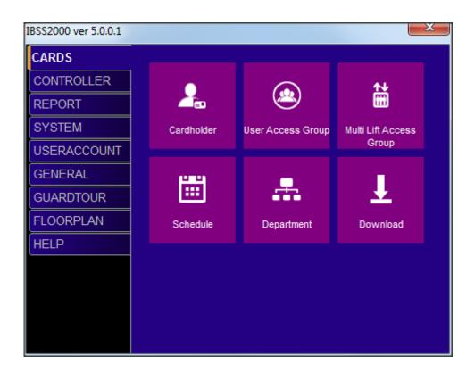
Multi Lift Access group configure ACU1000 output zone to be assign to a group (Multi Lift Access Group). 255 groups is support in a system.
