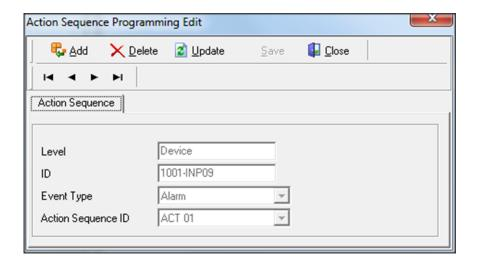
Action Sequence work in real time, meaning Commsvr need to be online for Action Sequence to function.
