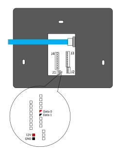
Terminating AFR8630 to ACU controller is using 2 set of cable, Power cable (12V, GND) and Wiegand data cable (Data 0, Data 1). LAN cable is optional but critical when using Central Enrolment. LAN cable is directly connected to Network Switch. The recommended extension cable is Belden 9538 24AWG 0.6mm 8 core cable foil shield.
