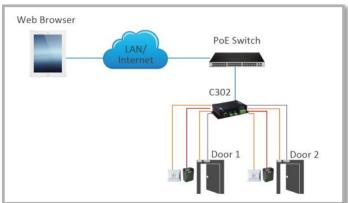
Standalone IP Controller with Door Module Configuration
